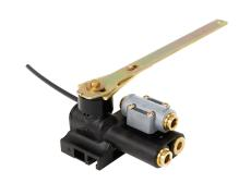
Cross Flow Valve Instant Response Valve Variable air flow rate with Dump Facility 3/8" Push to connect (PTC) air supply ports 1/4" Push to connect dump port 150psi max operating pressure VALVE ONLY
