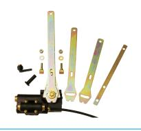
Instant Response Valve Variable air flow rate with Dump Facility 1/4" Push to connect (PTC) air supply & dump ports 150psi max operating pressure **VALVE PLUS:** 1/4" elbow and 1/4"port plug 4 levers **Mounting bolts**
