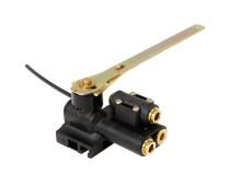
Instant Response Valve Variable air flow rate with Dump Facility 3/8" Push to connect (PTC) air supply ports 1/4" Push to connect dump port 150psi max operating pressure VALVE ONLY
